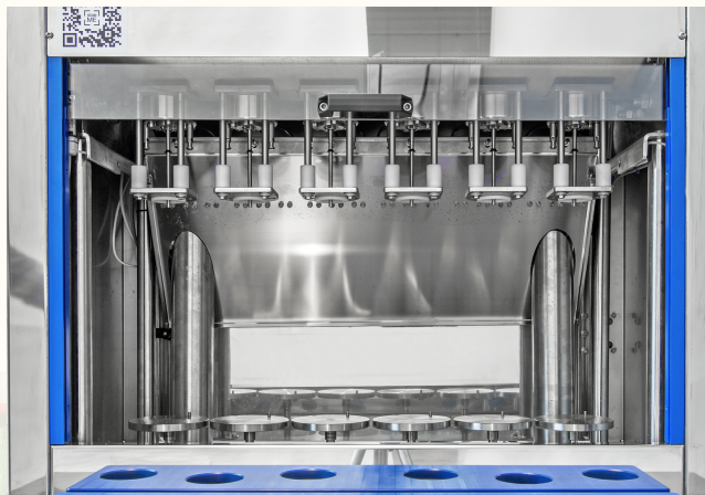
ISOBARIC FILLING UNIT WITH 6 ELECTROPNEUMATIC VALVES
