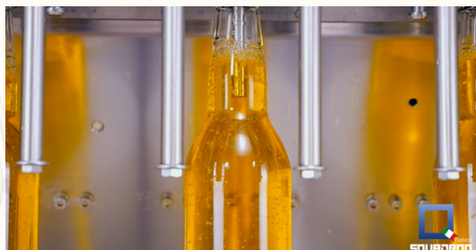
ISOBARIC FILLING UNIT WITH 6 ELECTROPNEUMATIC VALVES
